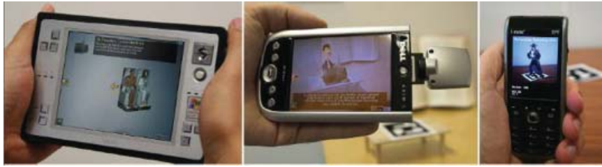
Figure 4. Examples of handheld mobile AR devices: UMPC, PDA, and SmartPhone (images courtesy of Wagner and Schmalstieg 17 ).
