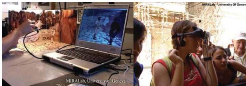
Figure 3. Example of a mobile AR system based on a laptop, backpack, and video see-through HMD (images courtesy of Papagiannakis et al. 71 ).
