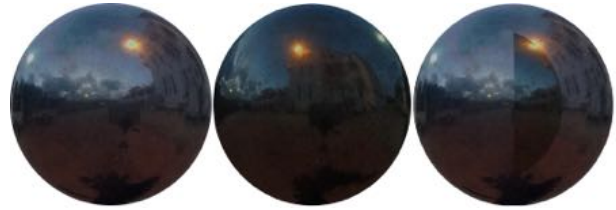
Figure 3: The captured HDR mirror ball images (left) and the generated final one (right)
